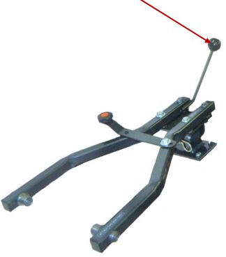
INSTALL KNOB ONTO HANDLE EXTENSION THREADED END
